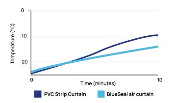
The temperature in the trailer with air curtain rises significantly slower during a 10 minute door opening.
